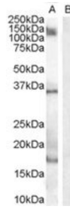
EB07174 (1µg/ml) staining of Human Peripheral Blood Mononucleocyte lysate (35µg protein in RIPA buffer) with (B) and without (A) blocking with the immunising peptide. Primary incubation was 1 hour. Detected by chemiluminescence.
