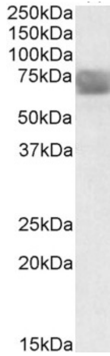
EB09574 (0.3 \mu g/ml) staining of Human Placenta lysate (35 \mu g protein in RIPA buffer) with (B) and without (A) blocking with the immunising peptide. Primary incubation was 1 hour. Detected by chemiluminescence.
