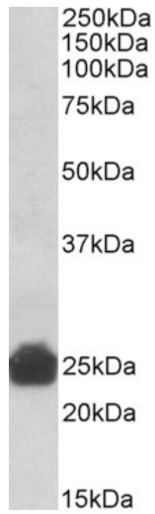
EB10727 (0.3 \mu g/ml) staining of Rat Liver lysate (35 \mu g protein in RIPA buffer). Primary incubation was 1 hour. Detected by chemiluminescence.
