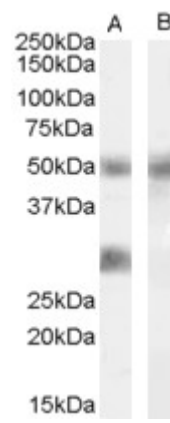
EB08005 (0.02µg/ml) staining of Human Breast Cancer lysate (35µg protein in RIPA buffer) with (B) and without (A) blocking with the immunising peptide. Primary incubation was 1 hour. Detected by chemiluminescence.
