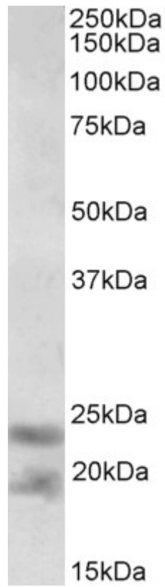
EB12023 (0.3 \mu g/ml) staining of Human Prostate lysate (35 \mu g protein in RIPA buffer). Primary incubation was 1 hour. Detected by chemiluminescence.
