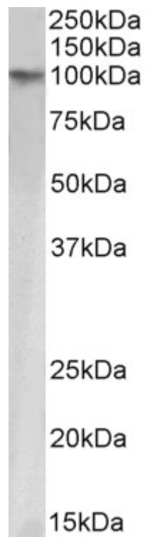
EB07662 (1 \mu g/ml) staining HeLa nuclear lysate (35 \mu g protein in RIPA buffer). Primary incubation was 1 hour. Detected by chemiluminescence.
