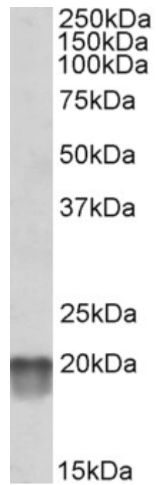
EB010191(0.1 \mu g/ml) staining of Human Heart lysate (35 \mu g protein in RIPA buffer). Detected by chemiluminescence.
