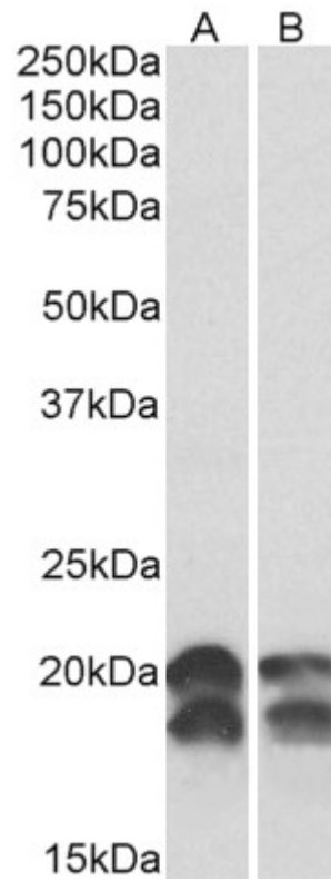
EB12579 (0.01 \mu g/ml) staining of A549 (A) and HeLa (B) lysates (35 \mu g protein in RIPA buffer). Primary incubation was 1 hour. Detected by chemiluminescence.
