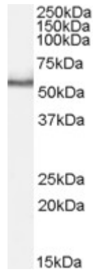
EB07940 (1 \mu g/ml) staining of Rat Testis lysate (35 \mu g protein in RIPA buffer). Primary incubation was 1 hour. Detected by chemiluminescence.
