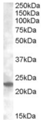
EB08314 (0.2 \mu g/ml) staining of Mouse Kidney lysate (35 \mu g protein in RIPA buffer). Primary incubation was 1 hour. Detected by chemiluminescence.
