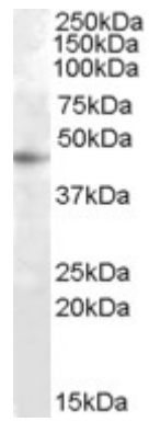
EB08394 (1 \mu g/ml) staining of HepG2 cell lysate (35 \mu g protein in RIPA buffer). Primary incubation was 1 hour. Detected by chemiluminescence.
