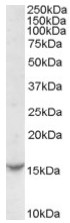
EB07720 (0.1µg/ml) staining of Jurkat Cell lysate (35µg protein in RIPA buffer). Primary incubation was 1 hour. Detected by chemiluminescence.
