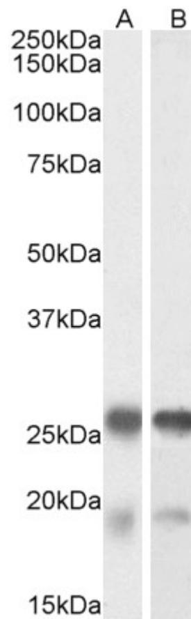
EB09800 (0.001 \mu g/ml) staining of Mouse (A) and Rat (B) Brain lysate (35 \mu g protein in RIPA buffer). Detected by chemiluminescence
