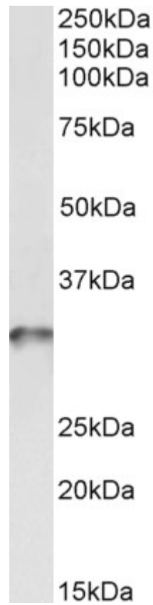
EB12417 (0.03 \mu g/ml) staining of Human Platelets lysate (35 \mu g protein in RIPA buffer). Detected by chemiluminescence.
