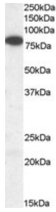
EB06268 staining (0.05 \mu g/ml) of Human Brain Cerebellum lysate (RIPA buffer, 35 \mu g total protein per lane). Primary incubated for 1 hour. Detected by western blot using chemiluminescence.
