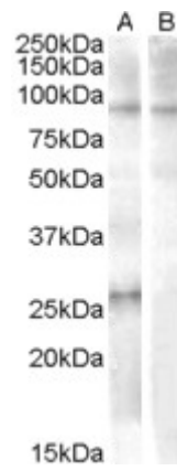
EB08357 (1 \mu g/ml) staining of Human Heart lysate (35 \mu g protein in RIPA buffer) with (B) and without (A) blocking with the immunising peptide. Primary incubation was 1 hour. Detected by chemiluminescence.
