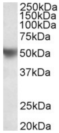
EB11195 (0.2 \mu g/ml) staining of Human Placenta lysate (35 \mu g protein in RIPA buffer). Primary incubation was 1 hour. Detected by chemiluminescence.
