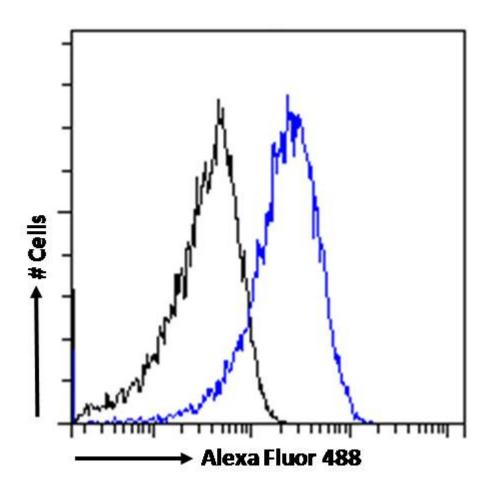
EB07557 Flow cytometric analysis of paraformaldehyde fixed A431 cells (blue line), permeabilized with 0.5% Triton. Primary incubation 1hr (10ug/ml) followed by Alexa Fluor 488 secondary antibody (1ug/ml). IgG control: Unimmunized goat IgG (black line) followed by Alexa Fluor 488 secondary antibody.
