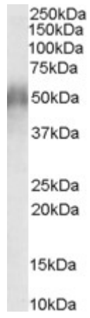
EB06414 (0.3 \mu g/ml) staining of Human Thymus lysate (35 \mu g protein in RIPA buffer). Primary incubation was 1 hour. Detected by chemiluminescence.
