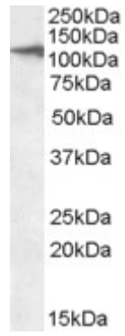
EB09210 (2 \mu g/ml) staining of Human Liver lysate (35 \mu g protein in RIPA buffer). Primary incubation was 1 hour. Detected by chemiluminescence.
