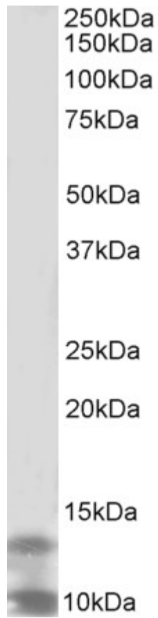
EB08946 (2 \mu g/ml) staining of K562 lysate (35 \mu g protein in RIPA buffer). Primary incubation was 1 hour. Detected by chemiluminescence.
