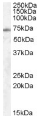
EB07225 (0.5µg/ml) staining of Human Lung lysate (35µg protein in RIPA buffer). Primary incubation was 1 hour. Detected by chemiluminescence.
