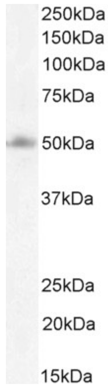
EB05608 (1 \mu g/ml) staining of U251 cell lysate (35 \mu g protein in RIPA buffer). Detected by chemiluminescence.
