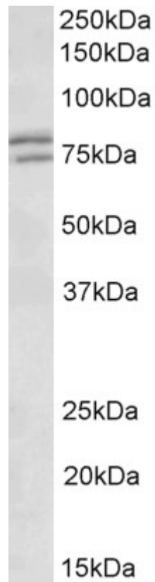
EB07361 (1 µg/ml) staining of NIH-3T3 cell lysate (35 µg protein in RIPA buffer). Detected by chemiluminescence.
