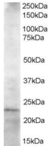
EB05750 staining (1.5 \mu g/ml) of Jurkat lysate (RIPA buffer, 35 \mu g total protein per lane). Primary incubated for 1 hour. Detected by western blot using chemiluminescence.
