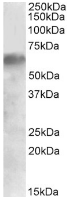
EB10698 (0.5 \mu g/ml) staining of Human Liver lysate (35 \mu g protein in RIPA buffer). Primary incubation was 1 hour. Detected by chemiluminescence.
