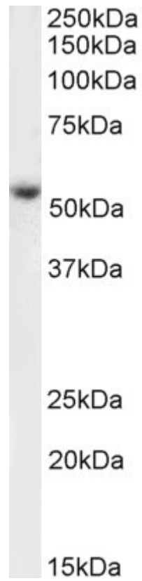
EB12988 (1 \mu g/ml) staining of Human Placenta lysate (35 \mu g protein in RIPA buffer). Primary incubation was 1 hour. Detected by chemiluminescence.
