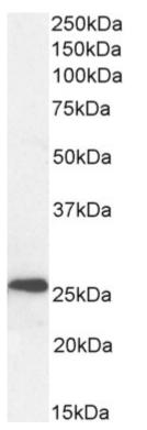
EB12057 (0.3μg/ml) staining of Human Spleen lysate (35μg protein in RIPA buffer). Detected by chemiluminescence.
