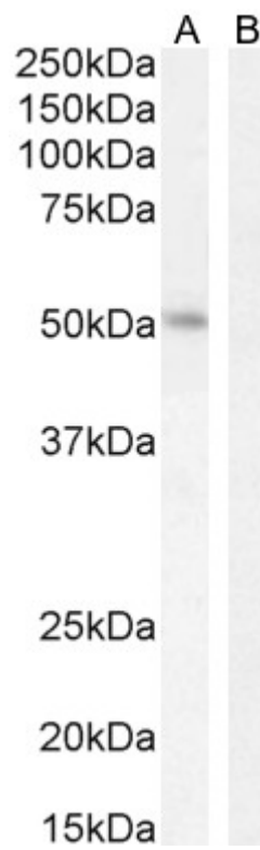
EB07196 (2 \mu g/ml) staining of K562 nuclear cell lysate (A) + peptide (B). (35 \mu g protein in RIPA buffer) Detected by chemiluminescence.
