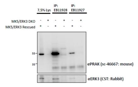
EB11927 and EB11928 (1.5ug) immunoprecipitations from lysates of MK5/ERK3 double knockout MEFs, with (third and fifth lanes) and without (fourth and sixth lanes) rescued MK5/ERK3 expression through retroviral transduction. The corresponding lysates (first and second lane resp.) were analyzed in parallel in this Western blot labelled with mouse anti-MK5 / PRAK (and co-precipitation was measured using rabbit anti-ERK3 in the lower panel).
