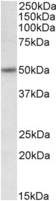
EB10833 (0.5µg/ml) staining of Mouse fetal Brain lysate (35µg protein in RIPA buffer). Detected by chemiluminescence.
