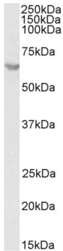
EB11523 (1 \mu g/ml) staining of K562 lysate (35 \mu g protein in RIPA buffer). Primary incubation was 1 hour. Detected by chemiluminescence.
