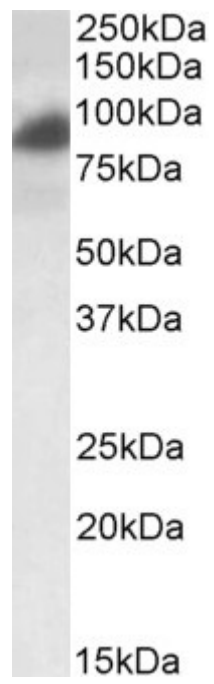
EB06897 (0.2 \mu g/ml) staining of HeLa lysate (35 \mu g protein in RIPA buffer). Primary incubation was 1 hour. Detected by chemiluminescence.
