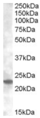
EB08314 (0.2 \mu g/ml) staining of Mouse Kidney lysate (35 \mu g protein in RIPA buffer). Primary incubation was 1 hour. Detected by chemiluminescence.
