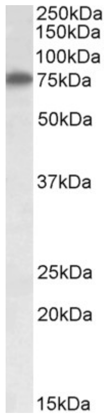
EB09780 (1 \mu g/ml) staining of HepG2 lysate (35 \mu g protein in RIPA buffer). Primary incubation was 1 hour. Detected by chemiluminescence.
