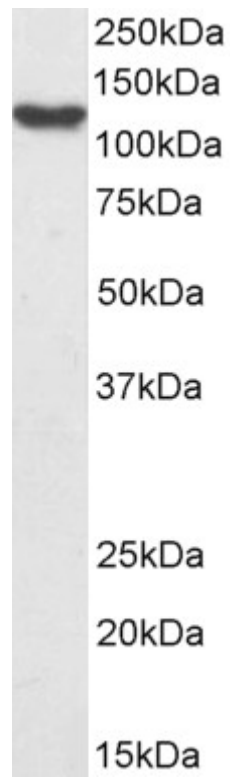
EB05441 staining (0.5 \mu g/ml) of HeLa lysate (RIPA buffer, 30 \mu g total protein per lane). Detected by chemiluminescence.
