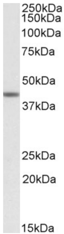
EB09594 (1 \mu g/ml) staining of Human Testis lysate (35 \mu g protein in RIPA buffer). Primary incubation was 1 hour. Detected by chemiluminescence.
