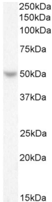
EB08892 (2 \mu g/ml) staining of Human Ovary lysate (35 \mu g protein in RIPA buffer). Detected by chemiluminescence.
