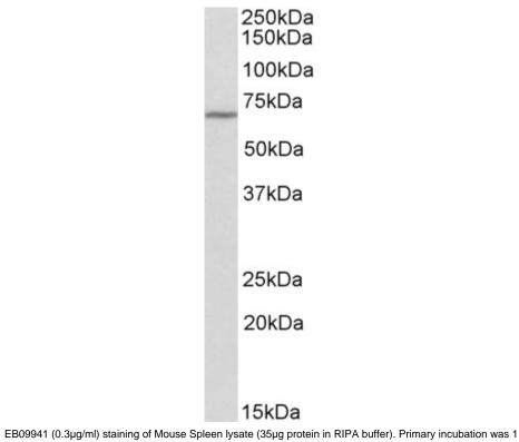
EB09941 (0.3µg/ml) staining of Mouse Spleen lysate (35µg protein in RIPA buffer). Primary incubation was 1 hour. Detected by chemiluminescence.
