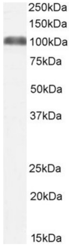
Western Blot: 0.1-0.5 \mu g/ml staining of Primary antibody in lysates EBL009-GPR94-G2, Approx. 100kDa band observed (calculated MW of 92.5kDa according to Human NP_003290.1). Primary incubation 1 hour at room temperature. Secondary antibody is EB2ND-002-A at 1:40K
